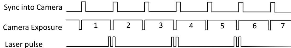
In the example above frames 1 to 6 will be stored in camera memory and contain the image pairs. If the laser cannot fire on all frames then some frames will not have illumination.
