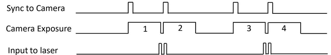
Using random snapshot allows only the frames required to be stored (no black non-illuminated frames) and therefore allows much longer samples of PIV double frames to be stored in the cameras memory.
